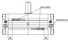
Note) For size 30, the auto switch cannot be mounted on the connection port side since there is a vacuum port.
