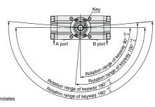
\* The shaft rotates clockwise when the pressure is applied from the A port while it rotates counterclockwise when the pressure is applied from the B port.
