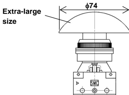
The button can be pushed with a palm, which reduces fatigue.
