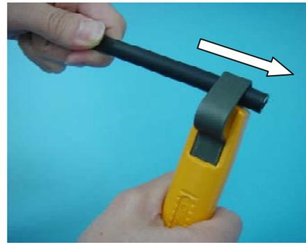
(2) Slide the tool longitudinally to cut into the outer layer (Note 1).
