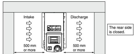
Note) The space must be 500 mm or more. Be sure that the ambient temperature is within the specification range.
