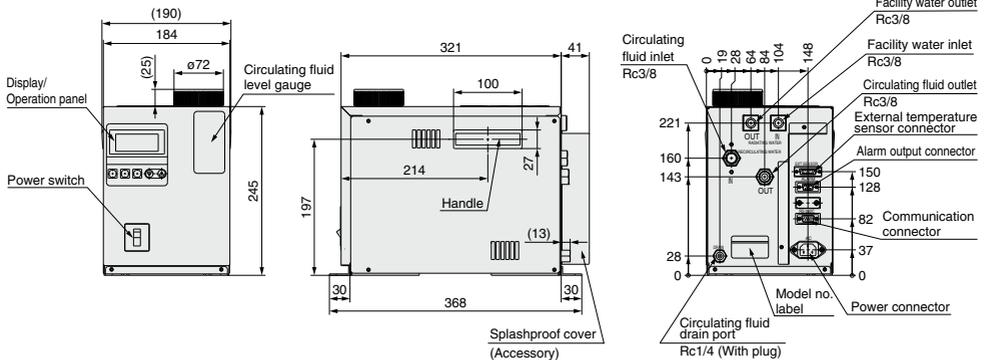
For NPT thread specification (-N), all fittings (including those at the circulating fluid drain port) are made of NPT.
