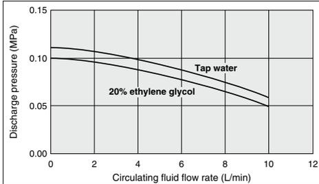
**HEC006** Since a DC pump is used, the unit is not affected by power requirements.
