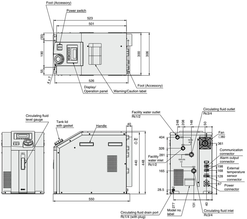
For NPT fitting specification (-N), all fittings (including those at the circulating fluid drain port) are made of NPT.
