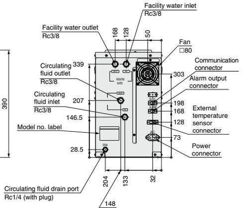
For NPT thread specification (-N), all fittings (including those at the circulating fluid drain port) are made of NPT.
